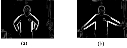
Fig. 6. Detected lines (bold and white) of human posture on the edge image. (a) Putting hands on the waist. (b) Stretching out the full arm.
