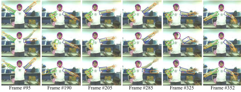
Fig. 14. Comparisons of tracking with different likelihood functions on a moving camera. (Top row: AMIS ; middle row: Color ; bottom row: Color + Edge .)
